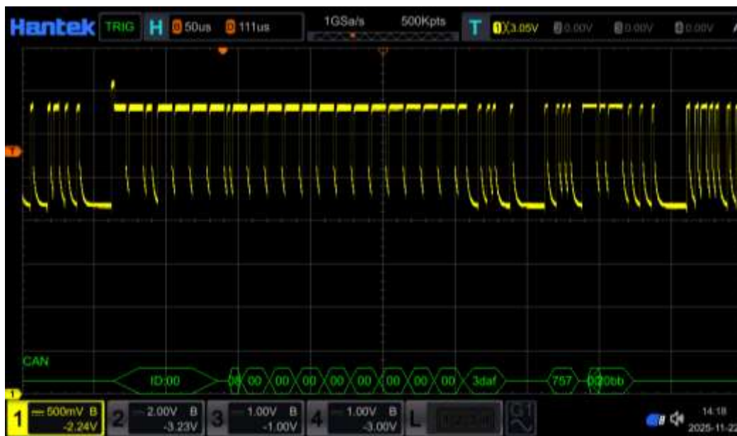
Figure 14.12 CAN Decoding example
