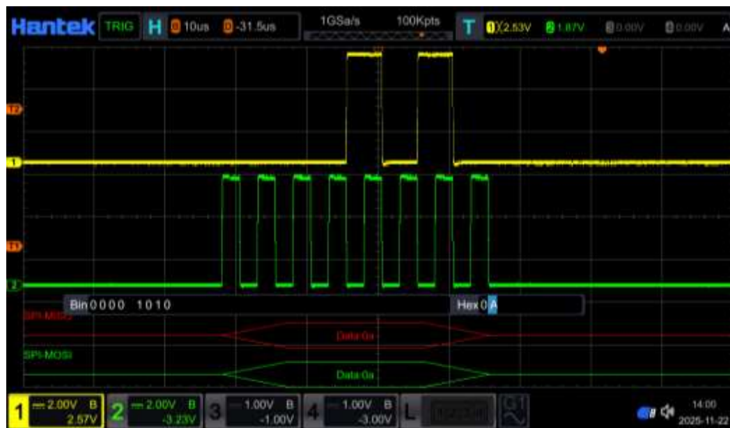
Figure 14.7 SPI Decoding example
