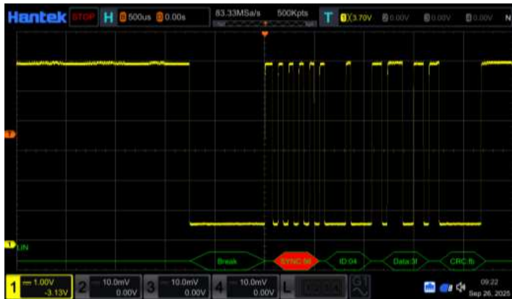
Figure 14.9 LIN Decoding synchronization error
