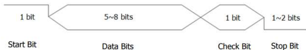
Figure 8.12 Schematic Diagram of UART Protocol
