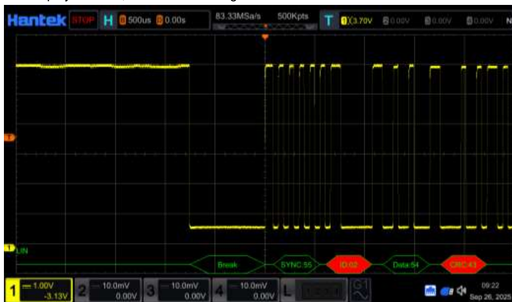
Figure 14.10 LIN Decode parity error
