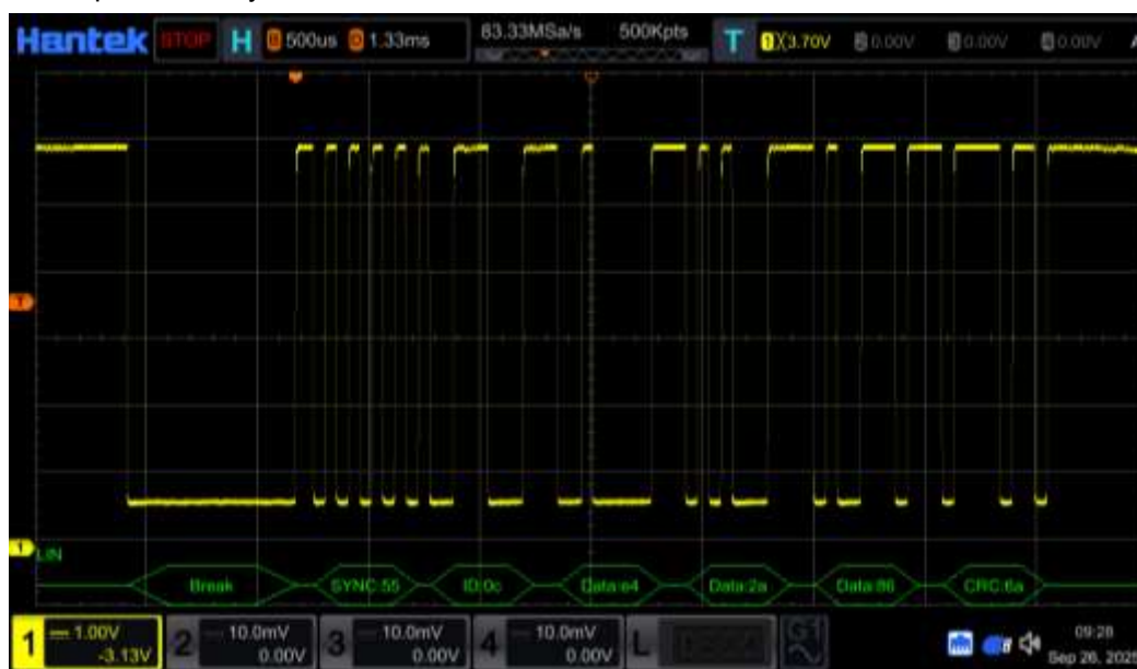
Figure 14.8 LIN Decoding example
