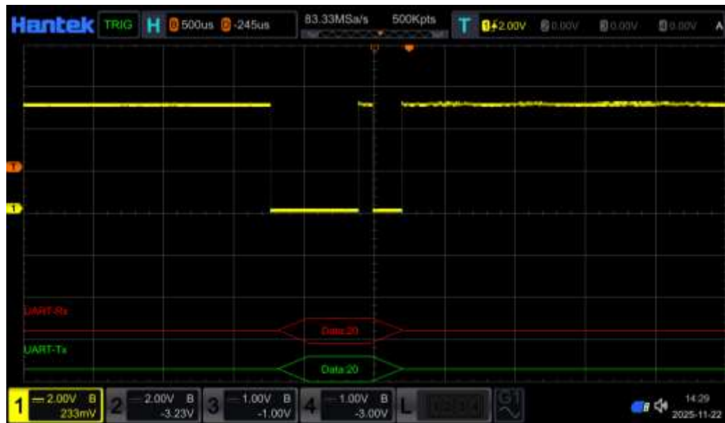
Figure 14.3 UART decoding example
