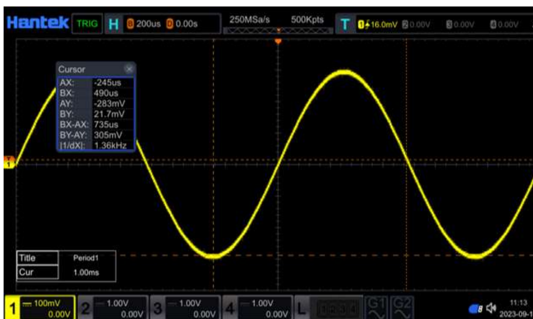
Figure 10.4 Track Measurement (after Horizontal Expansion)
